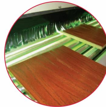
• **UV Flat Line Finishing** - Our flat line finish system offers great chemical resistivity, emits zero volatile organic compounds (VOCs) using solvent-free UV coatings.
