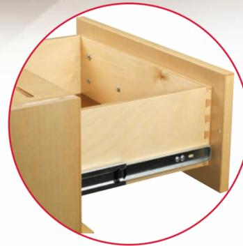
• **Dovetail Drawers** - Full height drawer sides are constructed with 1/2" thick 9-ply Baltic Birch with durable dovetail joinery at all four corners. Hardboard, melamine or veneered drawer bottoms are available options.
